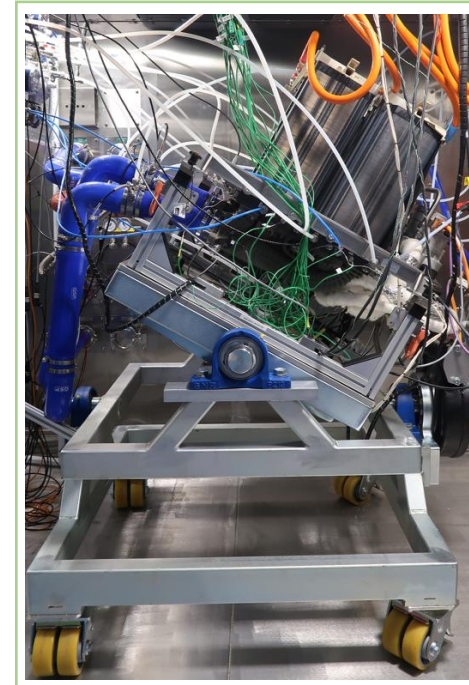
Twin stack inclination test
